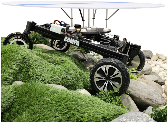
Fig. 1: COMPA demonstrating the ability to keep the turret horizontal (white plate) and directed (blue arrow), independent of the base pose, during holonomic off-road navigation.
