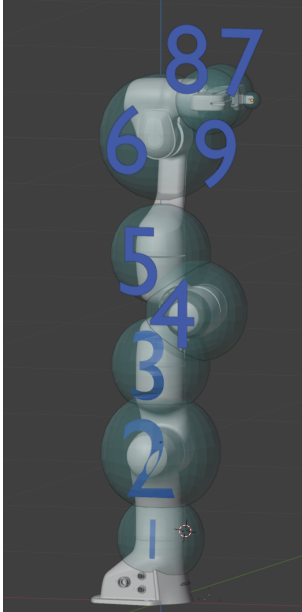
Figure 3: Spheres Hit-box Approximation
