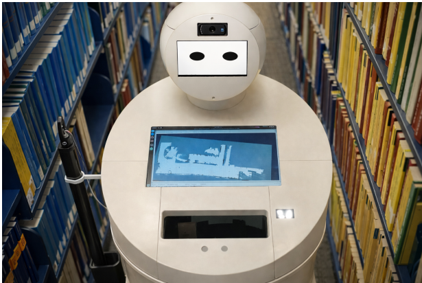
Fig. 4. Robot Mapping and Localizing Using SICK Picoscan 150
