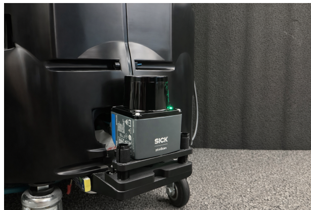
Fig. 3. SICK PicoScan 150 LiDAR mounted on the robot.
